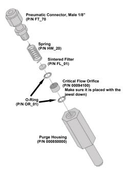
Figure 12-14: Critical Flow Restrictor Assembly/Disassembly
